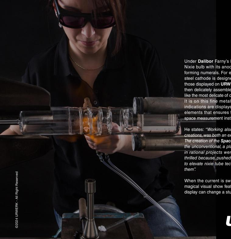
Under **Dalibor** Farny's brilliant guidanc Nixie bulb with its anodes arranged in forming numerals. For each unit display steel cathode is designed (the numerica those displayed on URWERK dials), i.e. 1 then delicately assembled element by ele like the most delicate of constructions. Eac It is on this fine metal spider's web t indications are displayed and it is the p elements that ensures the aesthetic ap space measurement instrument.
