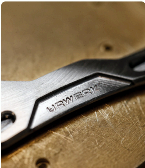
It will be treated with a PVD process to turn it black.
